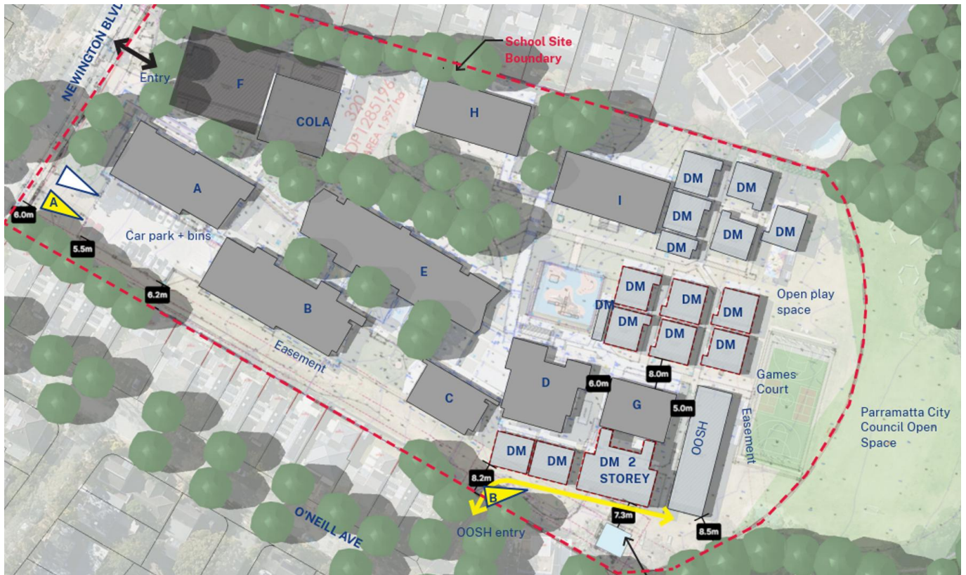
Figure 20: Construction access options
