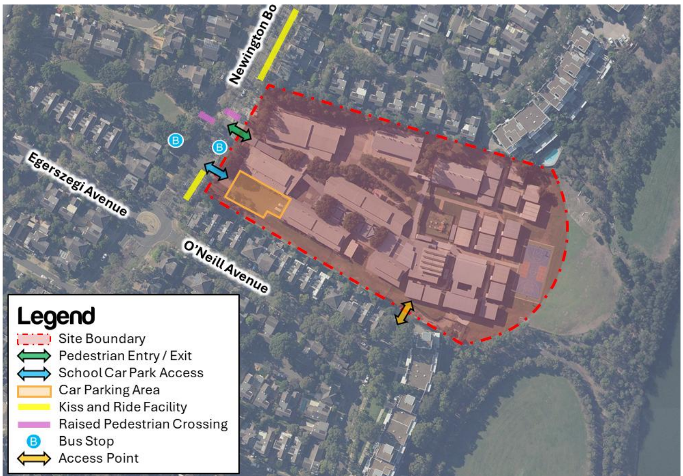
Figure 11: Pedestrian and vehicular access arrangements
