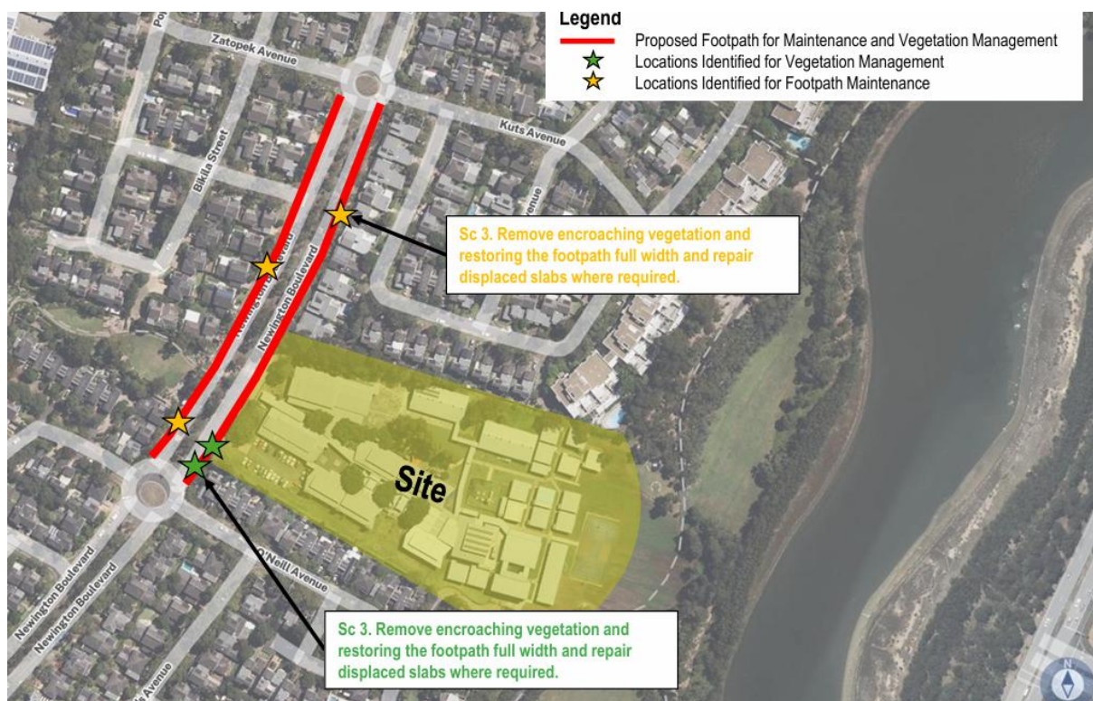
Figure 1 – Extract from the master plan showing the proposed footpath repair works and vegetation pruning works.
